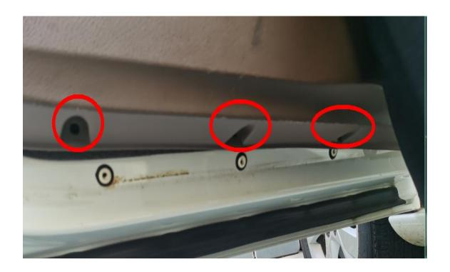
4-2. The outline light bar is pierced from the door frame and installed in the door gap. The construction is based on the door gap situation to avoid violent extrusion and explosion of the lamp beads.
