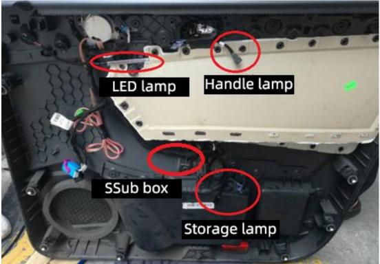
4-3. The handle light and the storage box light need to be installed by opening the hole. The opening position of the handle light is generally upward, and the position
